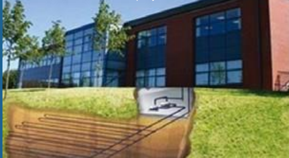
Horizontal Ground Loop System
