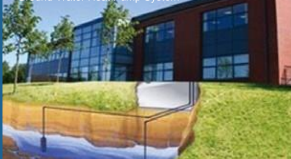
Ground-Water Heat Pump System
