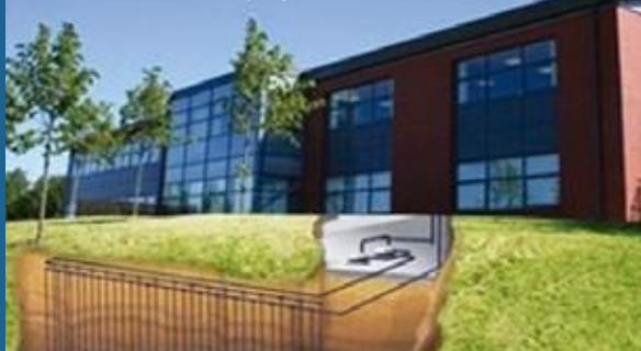
Vertical Ground Loop System
